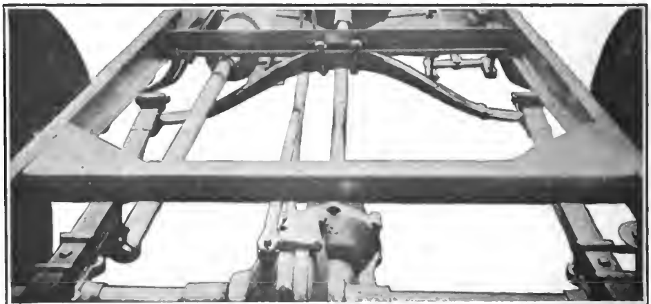
PLATFORM REAR SPRING SUSPENSION OF ST. LOUIS CARS. NOTE TRANSVERSE SPRING IS SHACKLED TO FRONT ENDS OF SIDE HALF ELLIPTICS.
